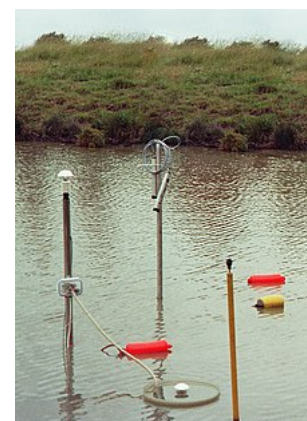
Instruments measuring condensation and evaporation at a Helmfleeth dew pond, 1970
