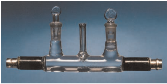
Figure 7 A cell for measuring fluid resistivity. Each end has a coaxial connection to a blacked platinum gauze electrode. There are two fluid ports for removing bubbles and a thermocouple well. The cell's geometric factor should be obtained by calibration with known fluids at each of the frequencies for which it will be used.
